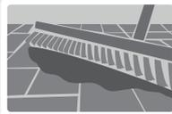
Using a **stiff nylon brush** apply the compound over the whole surface of the area being jointed.
