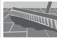
Once the water has been slightly evaporated, it is ready for a final **light brushing** to remove all the sand grains.
