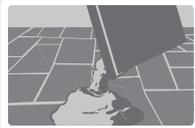
Clean the whole area to be pointed and **dampen the surface** then empty the compound on to the wet surface.
